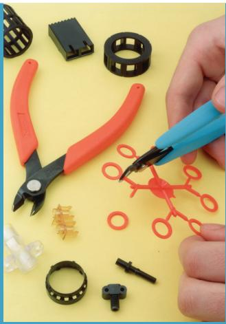
which can cause damage. The balance is dissipated into the opposing cutting edge of the cutter, which is why they get dull.
